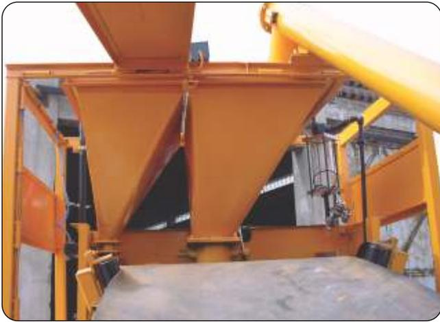
Individual weight hopper for cement, water and additive.
