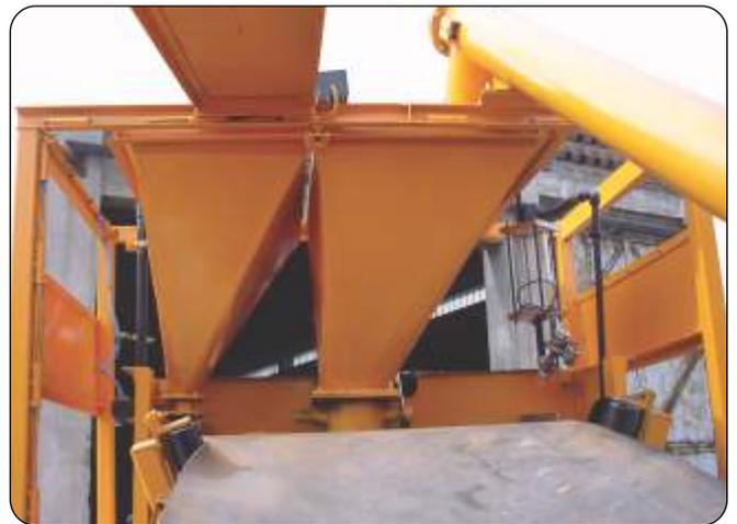
The plant has the complete features with a separate weigh hopper for Cement, Water and Additives which is weighed from weigh hoppers, screw conveyor of 5 mtrs length along with a ground hopper is provided for loading the cement.
