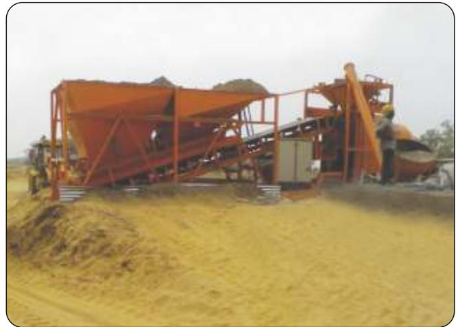
The plant needs very less space for storing and feeding cement of the cement fed directly in to the ground hopper which feeds into the cement weigh batcher through a screw conveyor. Minimum Work force is required for this operation.
