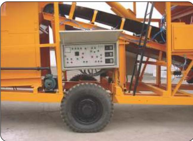
The control panel of the plant is fitted on the main chassis & is fully automatic and batching can be controlled through this panel. PLC based programme with touch screen and printing facility can be provided at an additional cost.
