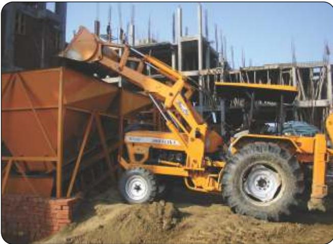
The portable plant has an advantage of being very user friendly, the aggregate bins can be loaded with a front end loader at ground level, minimum ramp is required for loading the bins. Thus requiring a very minimum space for installation of the plant.
