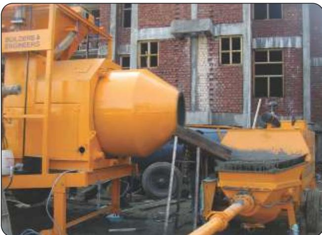
The main feature of this mobile plant is the mixed Concrete is discharged at a height of 1.5 mtrs, so as to enable dumping directly into the concrete pump.
